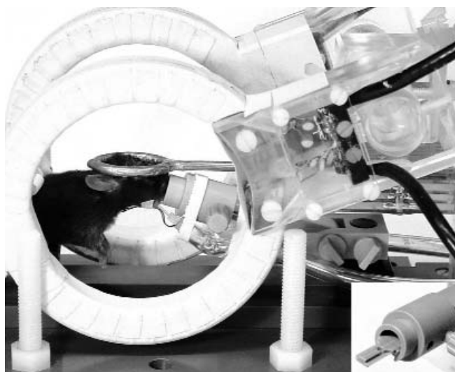
Fig. 1: Experimental set-up for MRI of mouse brain in vivo . Animals are intubated for inhalation anaesthesia and warmed by water-filled blankets. MRI signal excitation and detection is accomplished by use of a large Helmholtz coil (100 mm diameter) surrounding the whole animal and a small elliptical surface coil (20 mm anterior-posterior, 12 mm left-right) atop the head, respectively. The insert (right bottom corner) depicts the head holder comprising a nose cone and bite bar.
